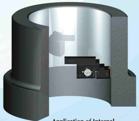
Application of Internal Roller Burnishing
